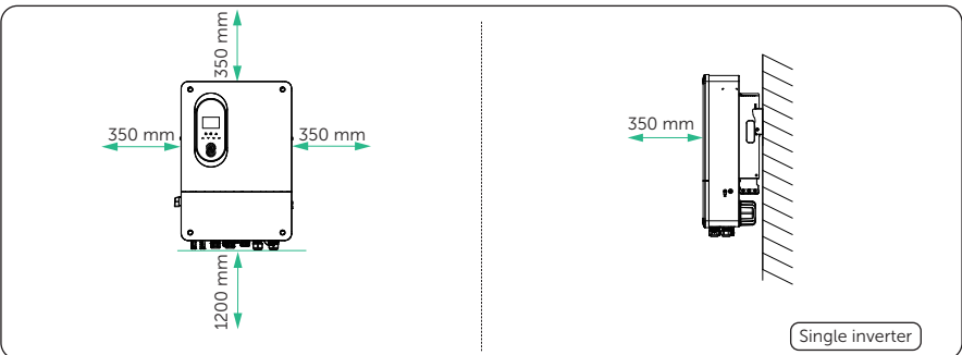
Figure 5-4 Clearance requirement for single inverter
